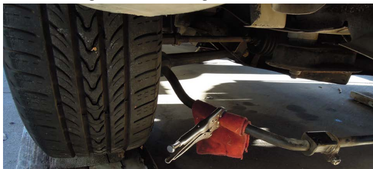
4. With a TR7 bar, you can just pull it out now. On a TR8, you can often muscle the bar out now too. But you can use a come-along if you're feeling fragile (like me). Two vice grips (with rags to protect the sway bar paint) and just 3 clicks on the come-along was all it took to get this one out. Voila!
