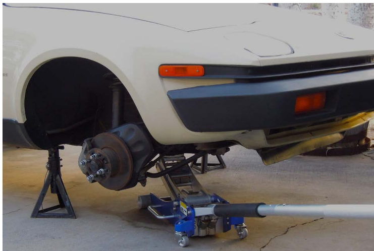
1. Jack up the car, support with jack stands, remove the wheels
