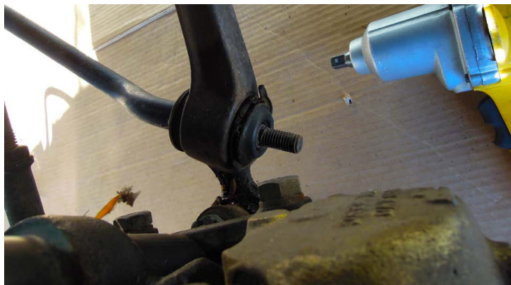
3. Remove the pins, washers, and nuts (above); the end bushings will come free later. Electric impact wrench (shown) for the end nuts is nice but not essential. Put the wheels back on, remove the jack stands and let the car down on its wheels (below). I used boards under the wheels to make it easier to get under the car. That compresses the suspension and makes sway bar removal easy!
