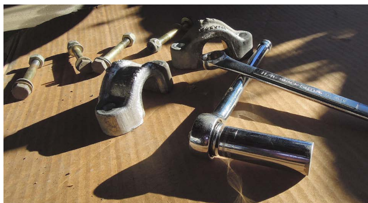
2. Remove the 4 nuts and bolts from the two anti-roll bar brackets and remove both brackets. I used a 17mm socket and 11/16" wrench to undo the bolts and nuts. The clamps (if you have them) can stay on the anti-roll bar.
