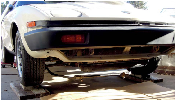
4. With a TR7 bar, you can just pull it out now. On a TR8, you can often muscle the bar out now too. But you can use a come-along if you're feeling fragile (like me). Two vice grips (with rags to protect the sway bar paint) and just 3 clicks on the come-along was all it took to get this one out. Voila!
