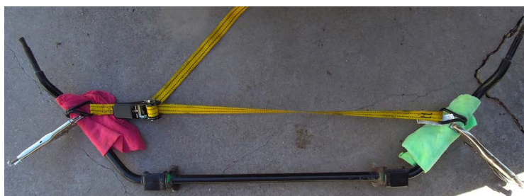
2. Remove the 4 nuts and bolts from the two anti-roll bar brackets and remove both brackets. I used a 17mm socket and 11/16" wrench to undo the bolts and nuts. The clamps (if you have them) can stay on the anti-roll bar.
