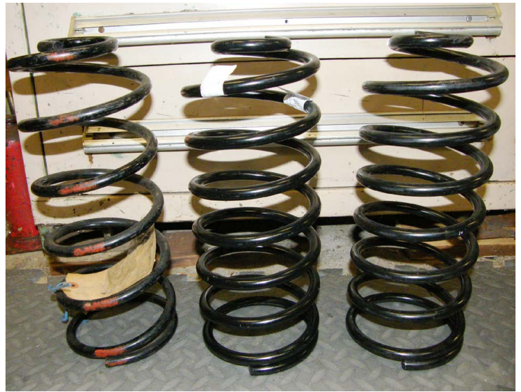
Original red stripe TKC1329 spring and two superceded GSV1029 replacements (which have too many coils)!
